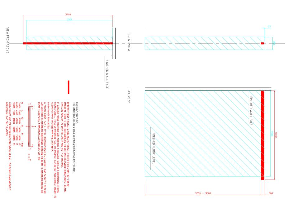
'REE ZONE FOR ROOF / WALL NO OBSTRUCTIONS IN THE MARKED ZONE, SUCH AS LIGHTING EQUIPMENT, HEATING STRIPS, VENTS, CABLES, ETC. PASS FROM FINISHED FLOOR LEVEL TO SOMM OF LINTELS.
